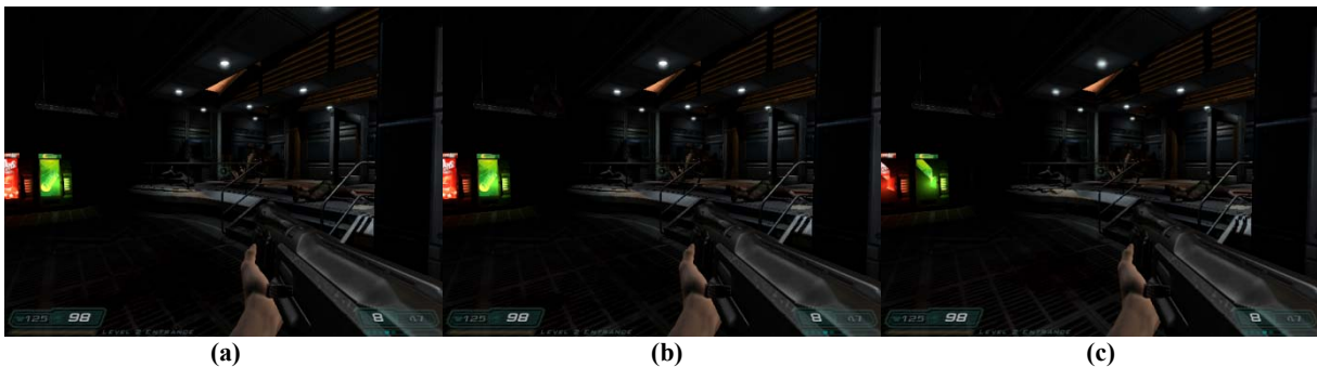
Fig. 1. Frame from the video game Doom 3 simulated at (a) full floating-point precision (24 bits per mantissa), (b) 19 bits, and (c) 16 bits of precision. The first two images are nearly visually identical, yet (b) saved 23% of the energy in the vertex transformation stage. While (c) exhibits a slight degradation in image quality, it saved 36% of the energy. Note that the slight loss of quality in 1(c) is due to errors in depth computation (known as “z-fighting errors”). These errors are sometimes present even in full-precision applications. When knowingly designing for a variable-precision video game, an artist could construct geometric models with care to avoid such errors.
