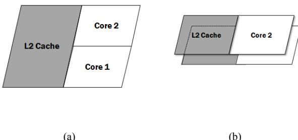
Fig. 2. (a) Planar layout of cores and an L2 cache, (b) 3D implementation of cores and an L2 cache
