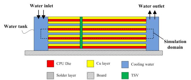
(b) Direct liquid cooling using water as a coolant
