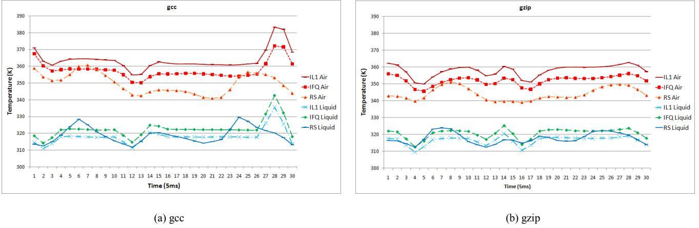
Fig. 5. Temperature comparison of three hottest functional units between the conventional air cooling scheme and the liquid cooling scheme.
