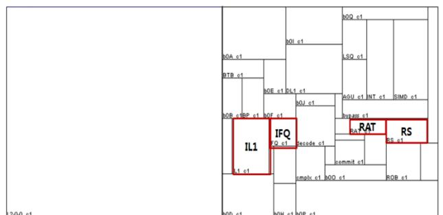
Fig. 3. Floorplan of a die in the 3D integrated processor.
