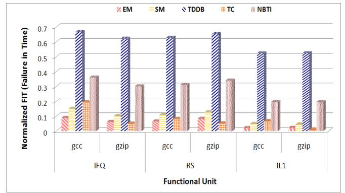
Fig. 7 Normalized FIT values for five different lifetime reliability models.
