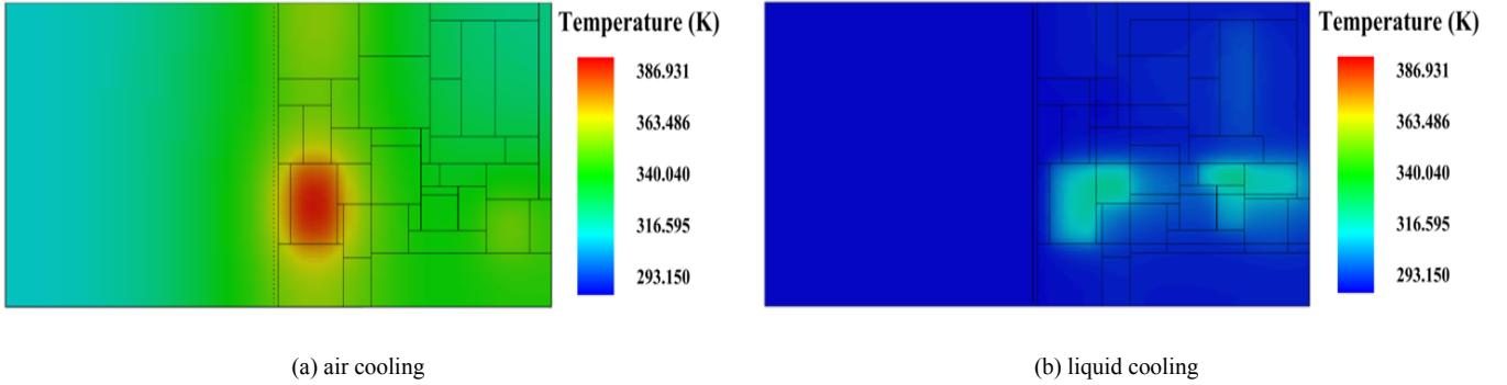
Fig. 4. Thermal profile of the 3D integrated processor (air cooling vs. liquid cooling)
