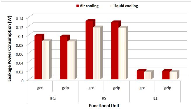
Fig. 6. Leakage consumption of the three hottest functional units.
